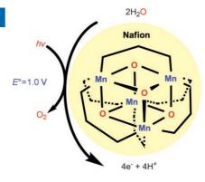
The generation game: A manganese–oxo complex with a cubic  $\{Mn_4O_4\}^{7+}$  core catalyzes the electrooxidation of water when suspended within the aqueous channels of a Nafion membrane (see picture). Illumination with visible light under an applied potential of 1.0 V (vs Ag/AgCl) generates current over one thousand turnovers. The catalytically active species arises from photolysis and subsequent dissociation of the manganese complex.
