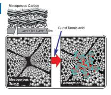
Tea or coffee? The layer-by-layer assembly of mesoporous carbon onto a quartz crystal microbalance results in a structure (see picture) that can be used for highly selective in situ measurement of nonionic aqueous guests, such as tea components.
