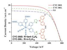
The sensitive type: Two new rutheniumbased supersensitizers (CYC-B6S and CYC-B6L) in which a hole-transport moiety and a conjugated segment are connected sequentially to the bipyridine of the ancillary ligand show efficiency in dyesensitized solar cells (DSCs) of up to 9.72%. Increasing the conversion efficiency of liquid-state DSCs by connecting a carbazole moiety to the ancillary ligand of the ruthenium-based sensitizer is demonstrated.
